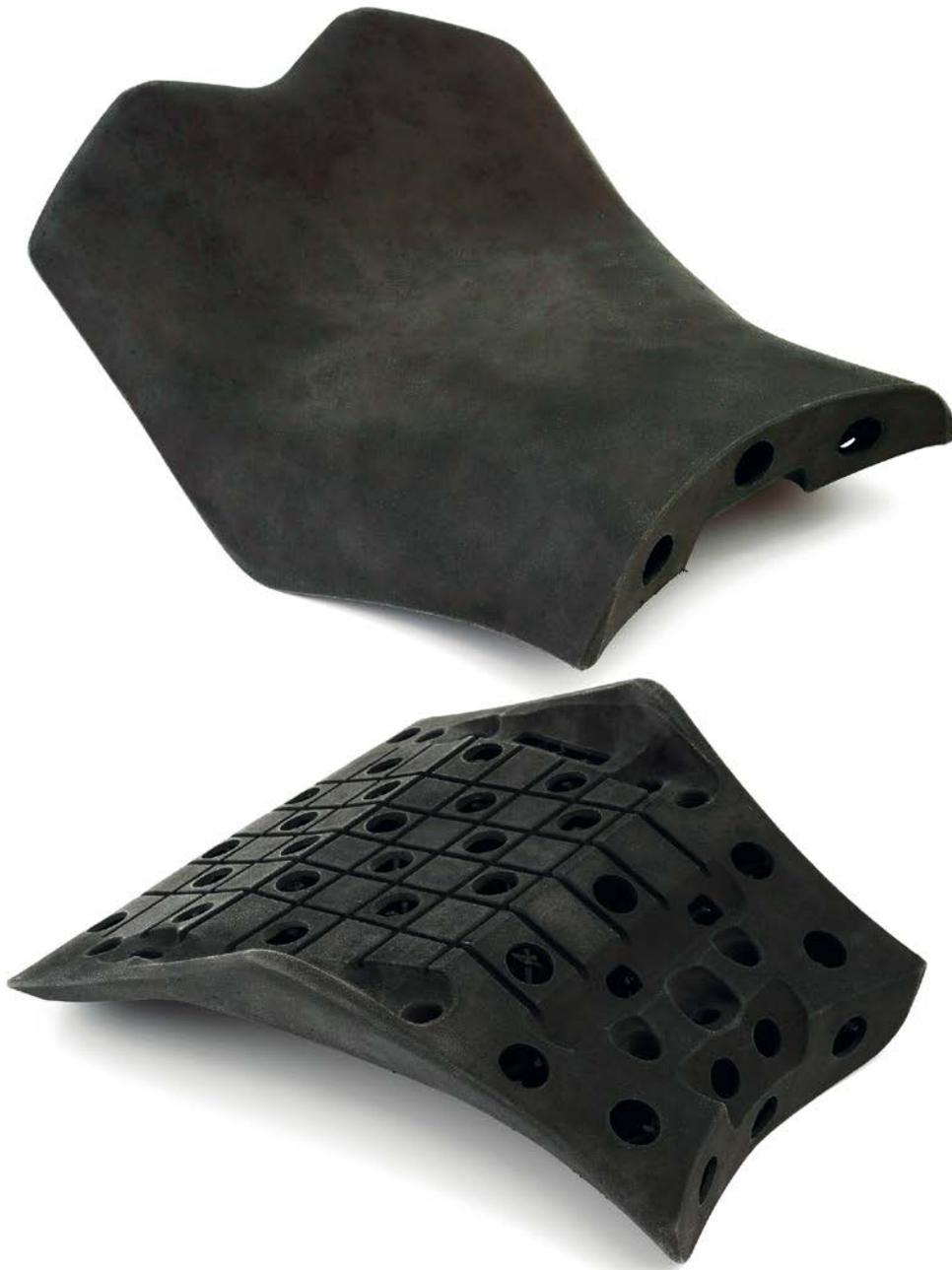
*Energica electric motorbike 3D printed seat with internal sandwich structure for customized pre-production series.
